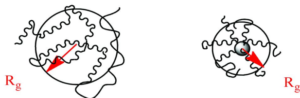
Figure 2. Schematic representation of the difference in root mean square radius of gyration of linear and star polymers of the same molecular weight.
